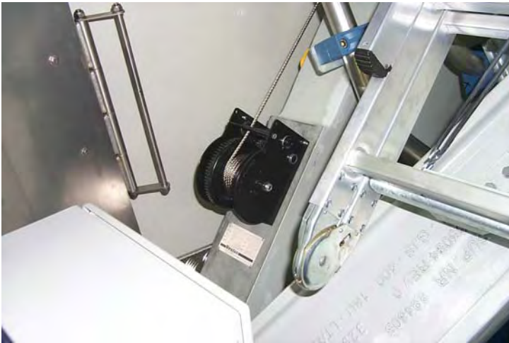
Figure 10 The Crane Winch placed on foundation.
